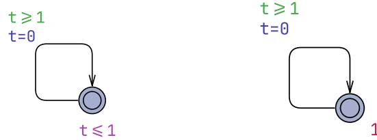
(a) Constant exact transition time of 1s (b) Exponential distribution of transition times with \lambda = 1
