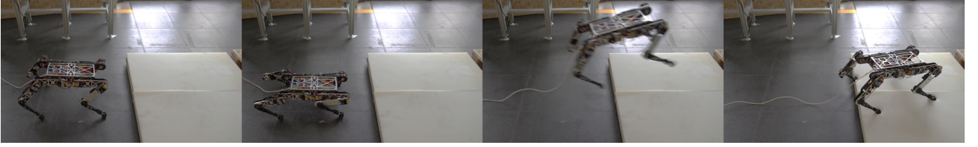
(b) Snapshots of the 10 cm jump experiment using Otto.
