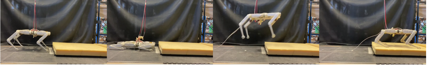
(a) Snapshots of the 7 cm jump experiment using Solo-12.
