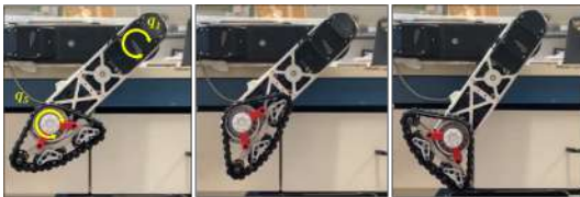
Fig. 10. The rotation of tracked actuator about hip joint ( q_1 ), and the rotation of the tracked foot about the ankle joint ( q_5 ). When the foot is lifted track orientation can be changed to approach an obstacle.
