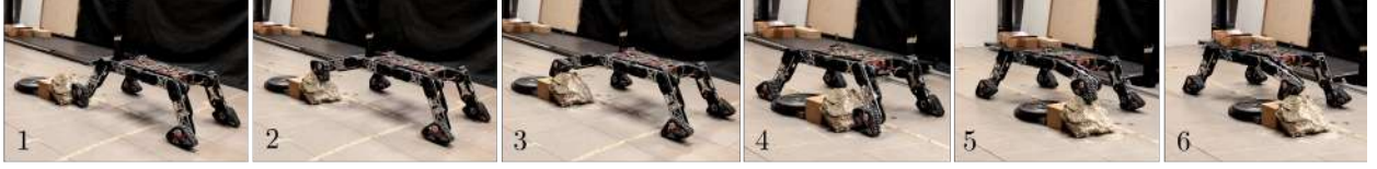
Fig. 16. TraQuad climbing a rock 1.75 times the height of its tracked foot and 50° slop using multi-modal locomotion. Phases: 1- LF track approaching the rock by opening the LF hip, 2- LF track is on the top of the rock while the hip is opened to accommodate the foot lift, 3- FL track is descending the rock by closing the hip. Similarly, 4- LH track approaching, 5- on top, and 6- descending the rock.
