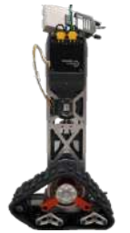
Fig. 8. Tracked foot assembly with EM-Act modular actuator.
