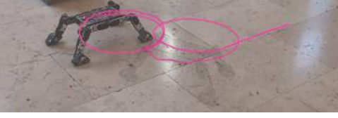
Fig. 12. TraQuad steering with tracked wheels (Turning radius = 0.25 m). The pink line showcases the tracking of the center of the robot's base link.
