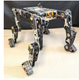
Fig. 24. The TraQuad II initial phase robot prototype (12-DOF). prototyped, the control system was developed, and the Stabil-iTrack algorithm was implemented to navigate and overcome structured obstacles and rocks. Successful demonstrations have highlighted the potential of multi-modal robots as essential solutions for overcoming challenging obstacles that uni-modal designs struggle with. Future work will focus on enhancing this design by incorporating a knee joint with an additional actuator in the leg. A 12-DOF version of this robot, named TraQuad II, is currently under development, with its preliminary design presented in Fig. 24.
