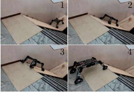
Fig. 13. TraQuad climbing a slope of 31^\circ using tracked wheels at a velocity of 0.9 m/s. Phases: 1- front tracks butt the inclined slope, 2 robot climbing on the slope, 3- front tracks reached the top corner of the slope, - rear tracks reached the top corner of the slope.
