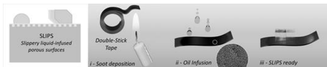
Figure 1. Cartoon showing the working principle and the fabrication procedure of SLIPs on tape.
