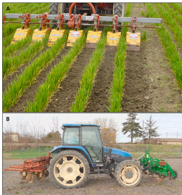
Fig. 1. Split rotary hoeing (SRH) during the devitalization of faba bean in alternate row temporary intercropping with wheat (A). Tractor with the complete roller multi-disk harrow (RMH): front-mounted machine for temporary intercrop management and rear-mounted disk inter-row cultivator (B).
