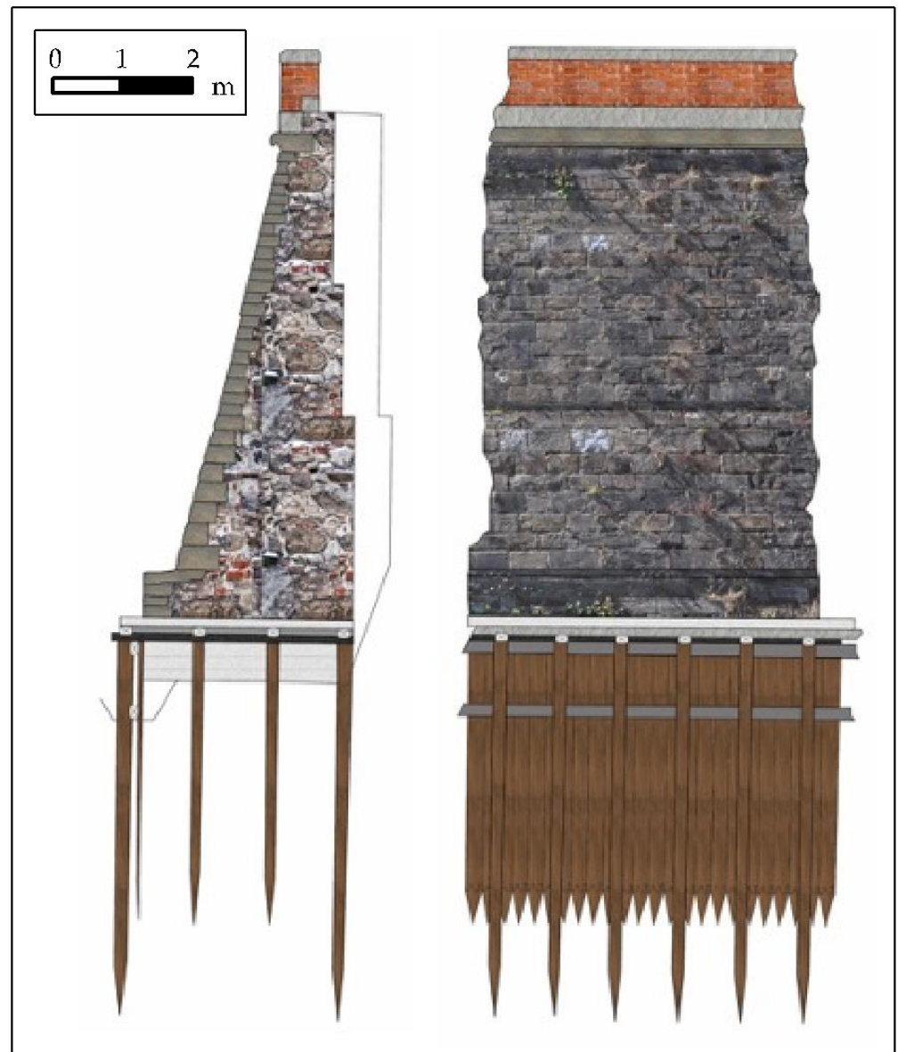
Figure 2. Construction techniques of the Lungarno Torrigiani riverbank (modified from original drawings preserved in the municipal historical archive of Florence).
