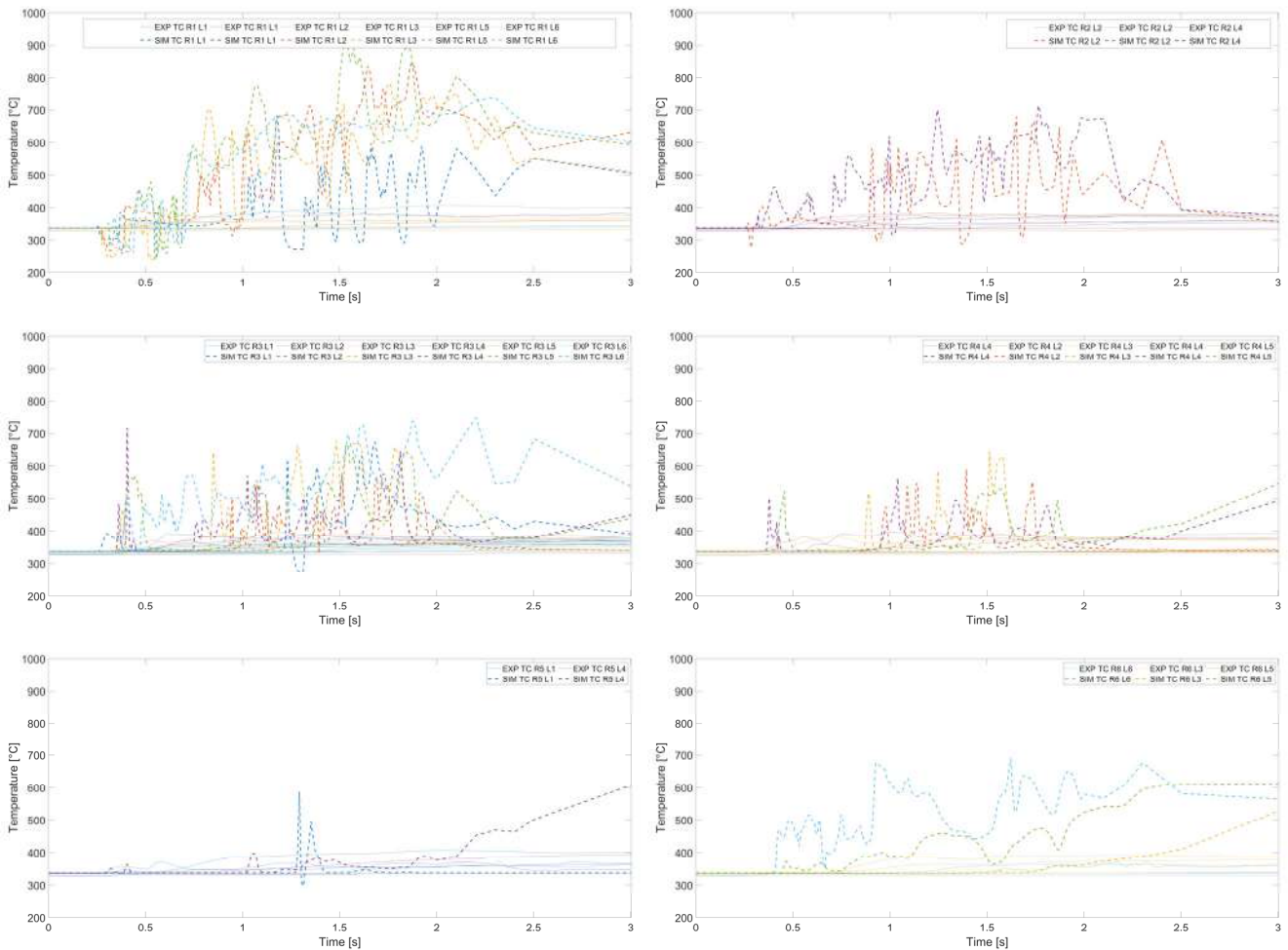
Figure 17. Temperature evolution in S1B for standalone simulations at different radial and axial positions (refer to Table 5).
