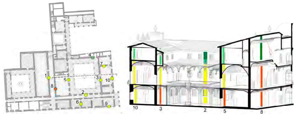
Figure 13. Visualization of the results of the safety assessment of walls in the ten sections (numbers 1–10) under gravity loads in the HBIM environment.
