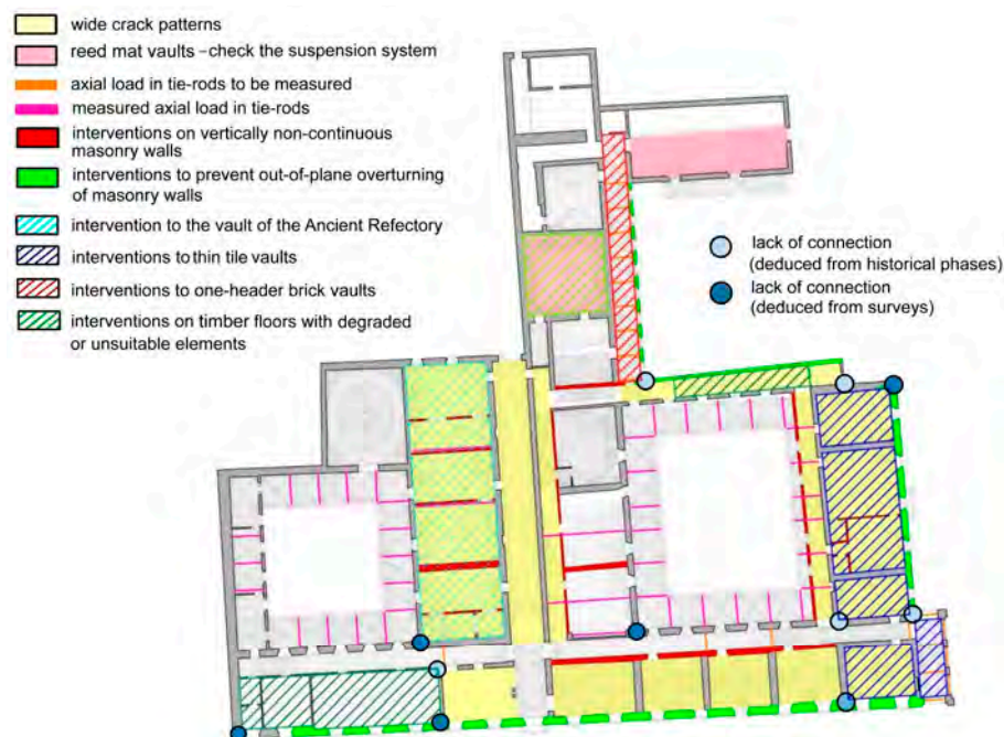
Figure 15. Plan of the second floor of the study area: the map summarizes the detected critical issues, the intervention categories, and the new knowledge needs.
