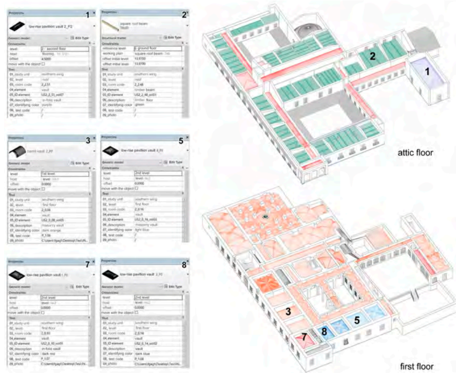
Figure 7. Views of the horizontal structures of the attic floor and the first level of the study area, with relative forms.
