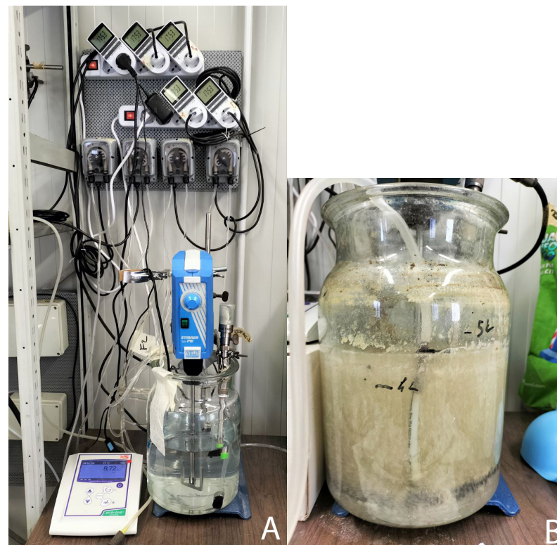
Figure 1. (A) Setup of the selection reactor: glass reactor with a stirrer, DO probe, pH meter, peristaltic pumps, aeration, and timed sockets; (B) Biomass inside the selection reactor during the famine phase.
