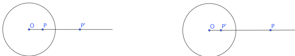
Figure 2. Inverse of a point P that is internal or external to the reference circle.
