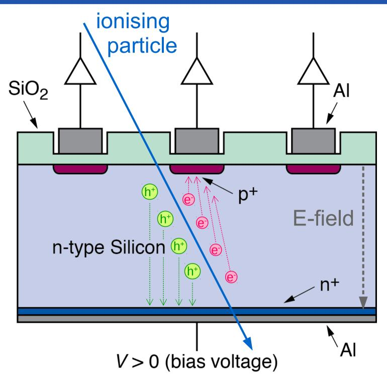
Silicon sensors are *pn* junctions operated in reverse bias mode. Charged particles create  $h^+e^$ pairs in a region depleted of thermal charge carriers by means of the applied bias voltage. Charges are then collected at the metal implant and read out. The mobility of the charge carriers depends on the magnitude of  $V_{bias}$ .
