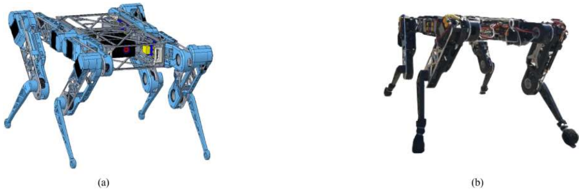
FIGURE 2. (a) CAD design of the Otto robot. (b) Otto robot.
