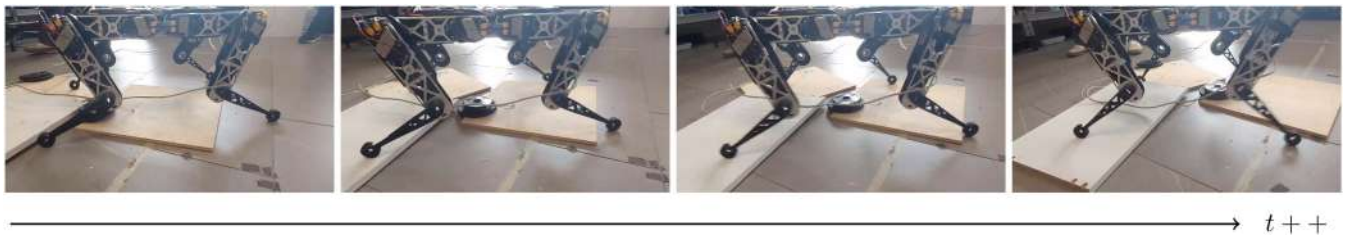
FIGURE 19. Photo sequence of Otto walking indoors with obstacles. Snapshots are taken within a 2-s window.
