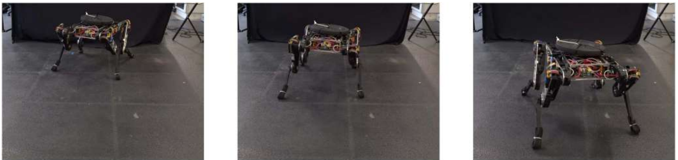
FIGURE 17. Photo sequence of the motion of the Otto robot while walking with a 5-kg payload.
