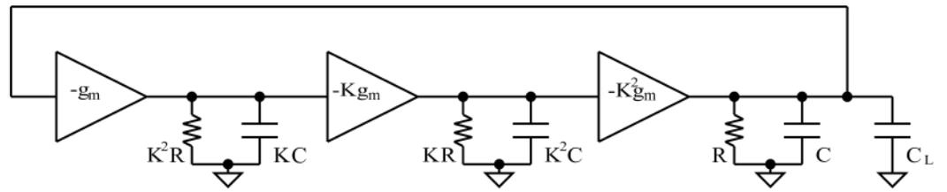
**Figure 1.** Model of a generic controlled oscillator based on asymmetric cells with a tapered factor  $K$ . The figure represents an RO-VCO with three cells, but it can be extended to a generic number of cells.
