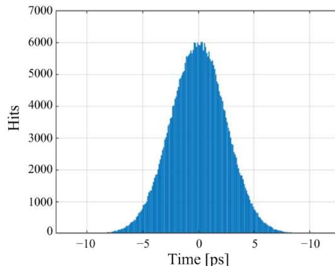
**Figure 11.** The cycle-to-cycle jitter histogram, measured with a 23 GHz 100 GS/s Tektronix mixed-signal oscilloscope evaluated at the target frequency of the RO-VCO.
