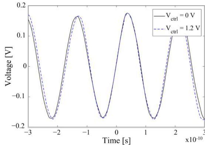
**Figure 10.** Image of the RO-VCO output signal measured with the oscilloscope: the black solid and the blue dotted traces were measured for the minimum and maximum RO-VCO control voltages, respectively. Both traces are triggered in the center of the graphic.
