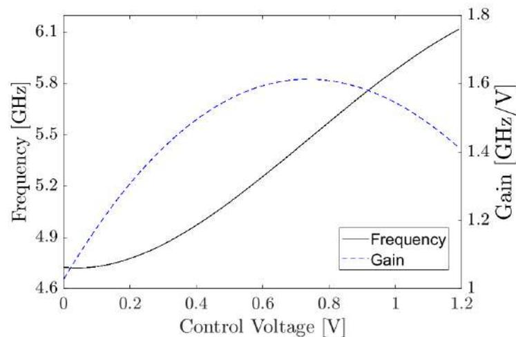
**Figure 9.** Measurement results of the proposed RO-VCO as a function of the control voltage: the black solid curve shows the free-running frequency, and the blue dotted curve represents the oscillator gain.
