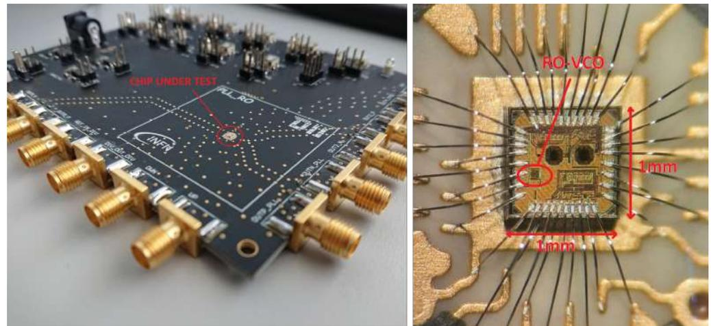
**Figure 7.** On the left, a photo of the high-speed board used for testing purposes. On the right, a microscope photo of the bare chip directly bonded with aluminum bonding wires on the high-frequency test board.
