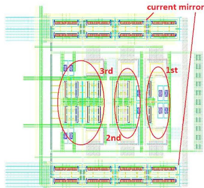
Figure 6. Layout of the proposed controlled oscillator.
