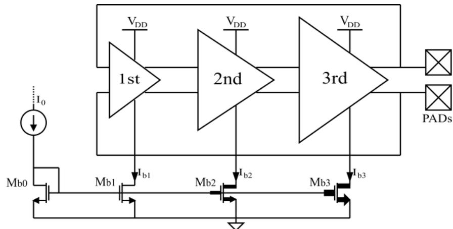
**Figure 3.** Electric schematic of the 3-stage differential and asymmetrical RO-VCO with the simple current mirror.
