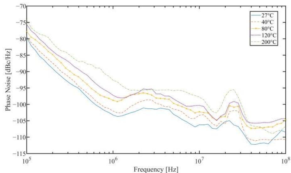
**Figure 13.** Phase noise measurements as a function of temperature between 27 °C and 200 °C. Around 2.5 MHz and 25 MHz from the carrier, an anomalous peak is observed, probably due to the COTS on the testing board used for the generation of the power supply and bias.
