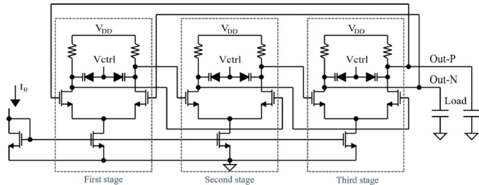
Figure 5. Whole schematic of the proposed three-stage RO-VCO.
