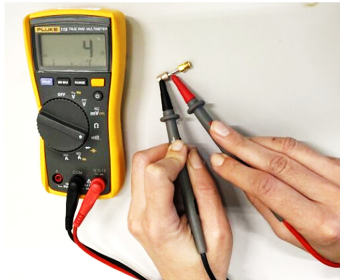
Figure 14. Laboratory test employing a digital multimeter to assess the electrical continuity between the metalized cylinder and the open-ended coaxial probe.
