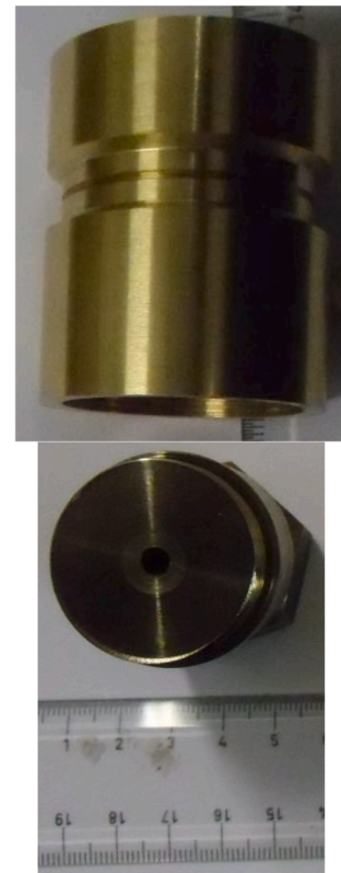
(b) View of the injection nozzle, orifice and the calibrated notched-section
