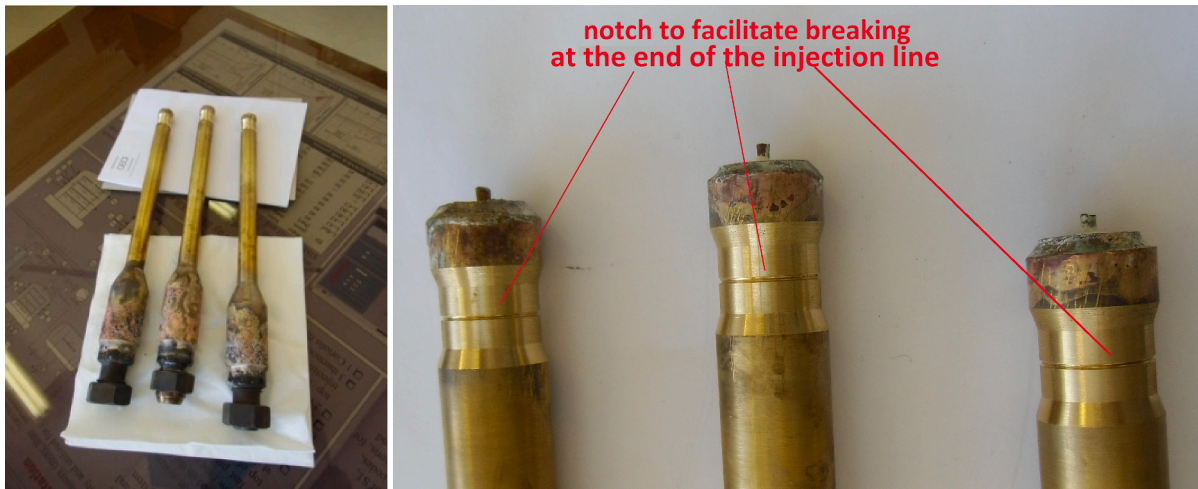
Fig. 13. LIFUS5/Mod2: view of injectors with protective caps.
