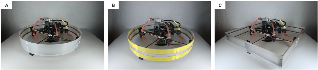
Fig. 8 | Three cages used during the experiments. A Streamlined, disc-shaped cage with low-friction shell. B Streamlined, disc-shaped cage with high-friction shell. C Non-streamlined, squared cage with low-friction shell.
