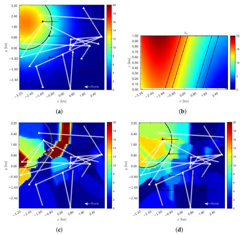
**Figure 4.** Rainfall rate estimation for a single realization with R=15 mm/h and  $g_{alg}=g_G=5$  mm/h/km. (a)  $\bar{\mathbf{r}}(\mathcal{C})$ :  $\pi_H(0)$  plane. (b)  $\bar{\mathbf{r}}(\mathcal{C})$ :  $\pi_V(y_G)$  plane. (c)  $\mathbf{r}(\mathcal{C})$ :  $N_{\text{CML}}=21$ ,  $N_{\text{BSL}}=0$ ,  $\varepsilon_{\text{RMS}}=5.715$ ,  $\rho=0.470$ . (d)  $\mathbf{r}(\mathcal{C})$ :  $N_{\text{CML}}=21$ ,  $N_{\text{BSL}}=8$ ,  $\varepsilon_{\text{RMS}}=1.981$ ,  $\rho=0.934$ .
