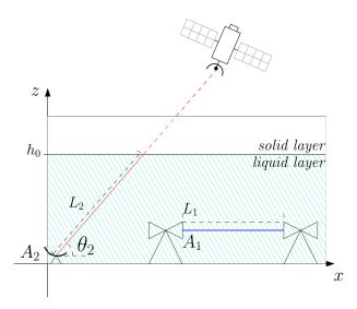
**Figure 1.** Stratiform rain model and geometry of the scenario. Link 1: CML, with length  $L_1$ , attenuation  $A_1$  and elevation angle  $\theta_1 = 0$ . Link 2: BSL, with wet path length  $L_2$ , attenuation  $A_2$  and elevation angle  $\theta_2$ .
