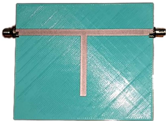
FIGURE 3 Picture of the fully 3D-printed T-resonator
