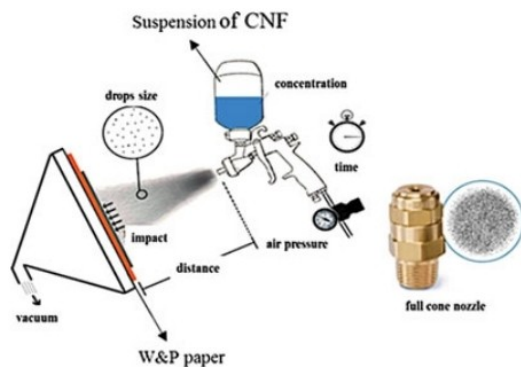
Figure 9. Scheme of the experimental procedure used for spray coating on paper with cellulose nanofibrils (CNFs) suspension. Reproduced from ref. [179] with permission from Taylor & Francis Group.
