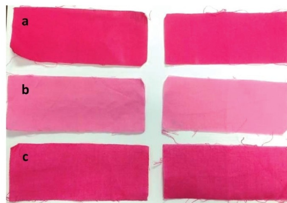
Figure 15. Cotton fabrics colored by using (a) a conventional exhaust dyeing method, (b) an exhaust dyeing method with a lower concentration of salt and alkali, and (c) the NFC-based dyeing method. Fabrics before (left column) and after (right) the accelerated laundering test (AATCC 61-2013, 2 A) are shown side by side. Reproduced from [207] with permission from the Royal Society of Chemistry.
