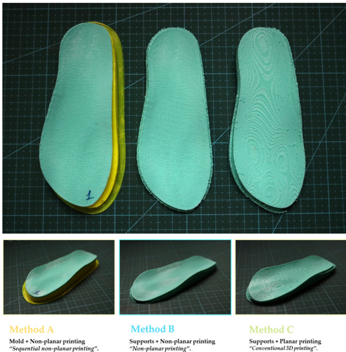
Figure 3. Prototypes for eco-impact assessment fabricated employing alternative printing strategies: methods A (left images), B (central images), and C (right images).
