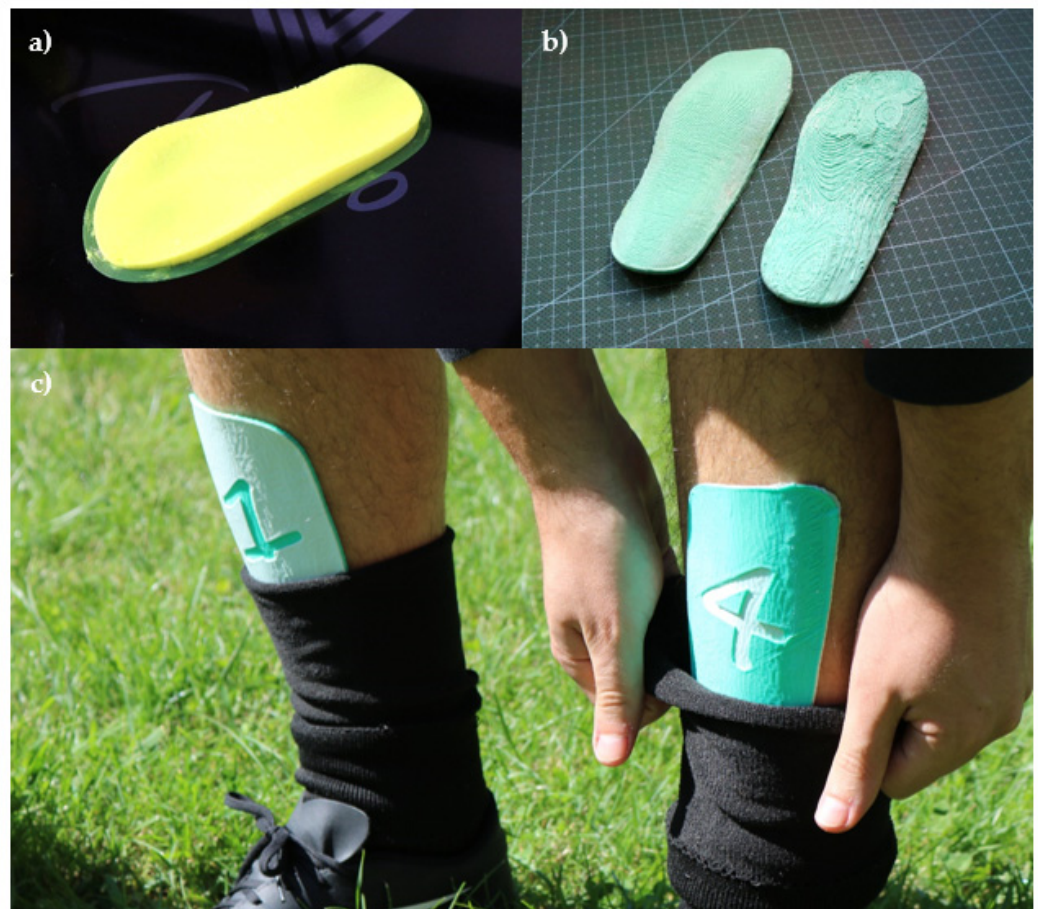
Figure 5. (a) Detail of supporting tool or printing mold after part detachment. (b) Surface aspect after printing and detachment from printing tool (left photo) and from conventional supports (right photo). (c) Alternative application case using similar processes: shin guards obtained employing non-planar printing with filaments of different colors for lower and upper layers, to enhance visual appeal.
