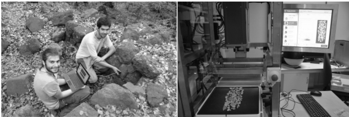
Figure 1. The Viavi micro probe used for recording spectral data on structures discovered during survey in Auvergne, France (on the left). The Sisuchema Pushbroom hyperspectral camera in the laboratory at Umeå University while scanning Mesolithic quartz tools (on the right).
