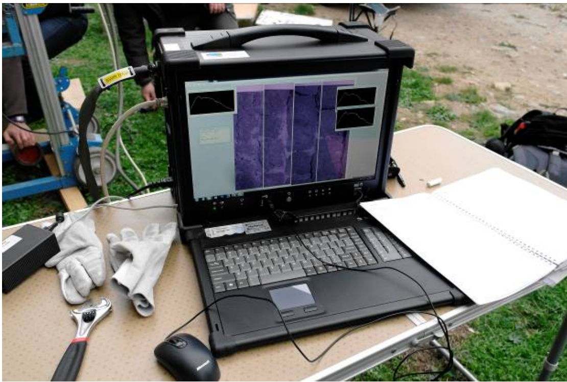
Figure 2. SWIR images visualized on the laptop in real time during data acquisition (Carcassonne project)
