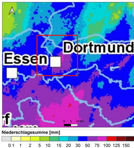
Fig. 8. Cumulated rain on the test area (square box) from July 14, 2021 05:50 UTC, to July 15, 2021 05:50 UTC, obtained from a weather radar [14].
