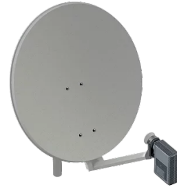
Fig. 2. IoT FIRST two-way terminal: 80-cm satellite dish and IST [7].
