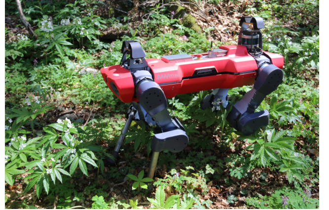
Fig. 3. ANYmal-C is a quadrupedal robot equipped with cameras, depth sensors and a LiDAR, enabling it to autonomously locomote in rugged, unstructured environments.
