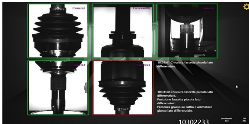
Fig. 14 Cell operator's GUI on a touch screen on the inspection station at the end of the robotized assembly cell. Inspection of clamp differential side closure, positioning, lubricant for the part number
