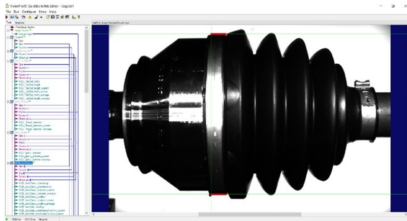
Fig. 15 A screenshot of the commercial vision software adopted. The block structure of the developed inspection software is shown on the left side. Right side provides an edge detected in red for the clamp under inspection
