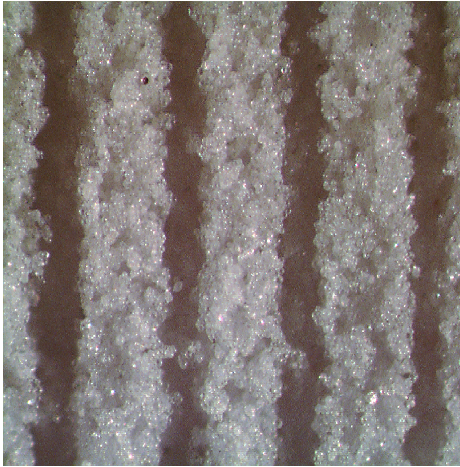
Figure 27 - Bed of 20 \mu\text{m} Alumina powder coated with a 10% solution of Duramax 3007. Clusters of 5-6 grains denote a sticky bed
