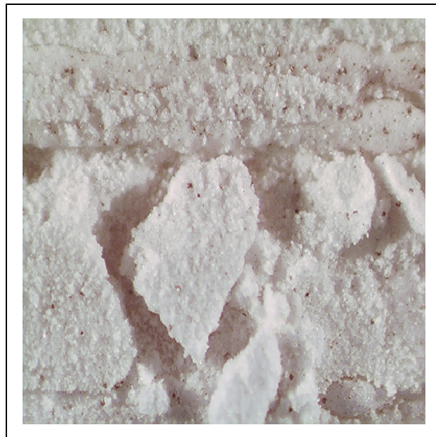
Figure 30 - Bed fragments show the strong forces among grains. The lines are poor. With 20% 5 \mu\text{m} tapping
