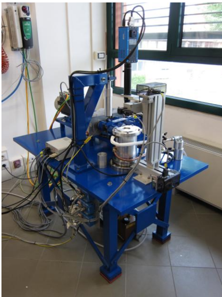
Figure 1 Pictures of the test rig for cam-follower pairs
