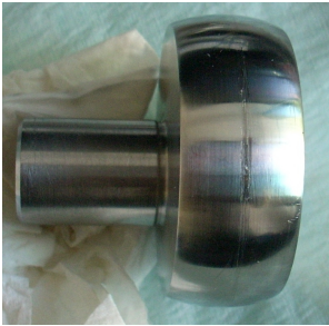
Fig. 9 – After tests picture of the specimen. Wear marks around 180° angular position.
