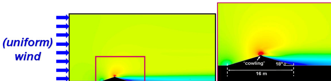
Fig. 4. dimensions of the simplified domain, and velocity field.
