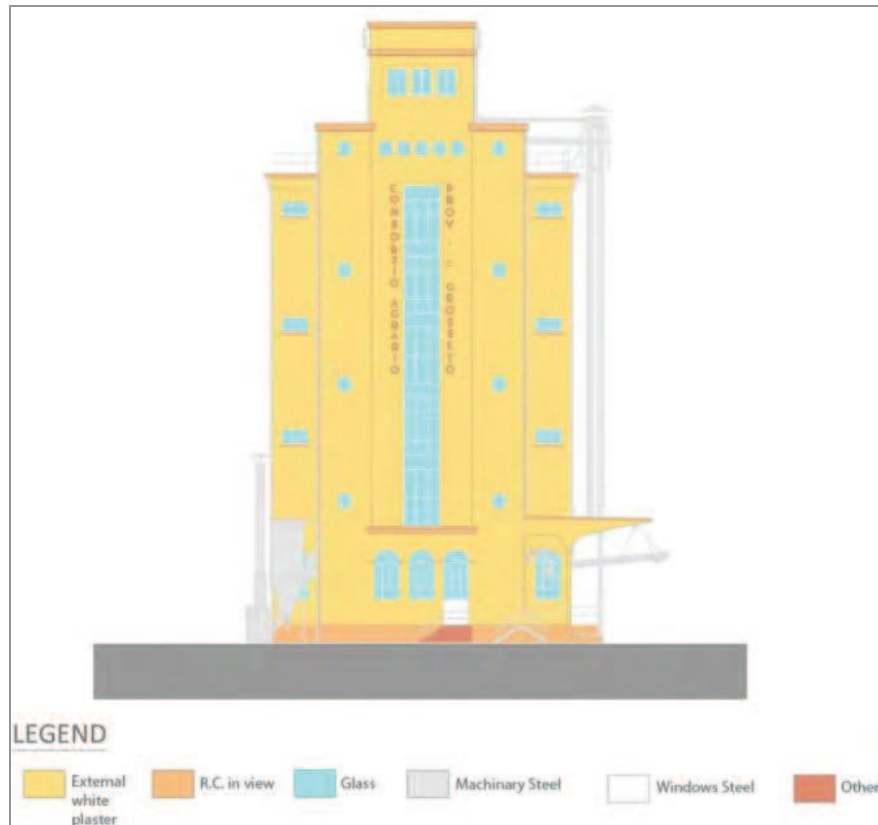
Figure 18 Example of building materials survey: the main façade
