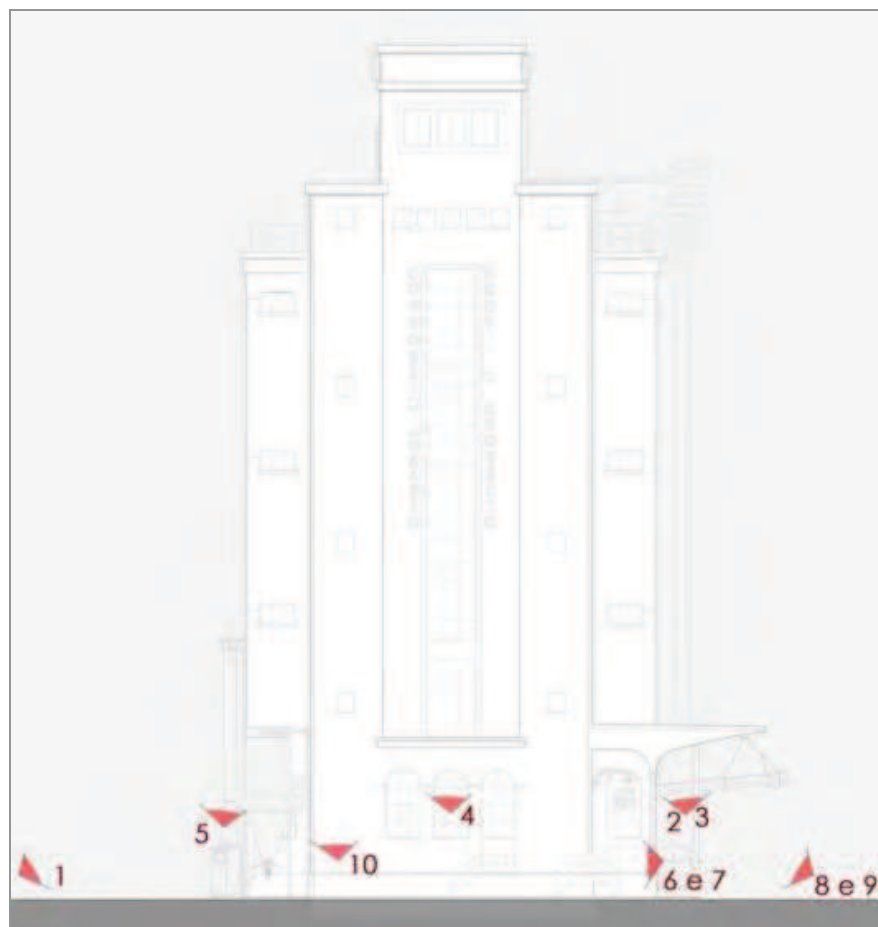
Figure 19 Example of decay survey: the main façade
