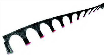
Figure 56 The second mode shape of the structure
