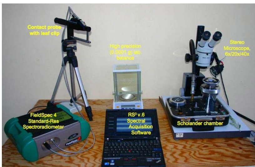
Fig. 1 - Experimental setup used during the research activity
