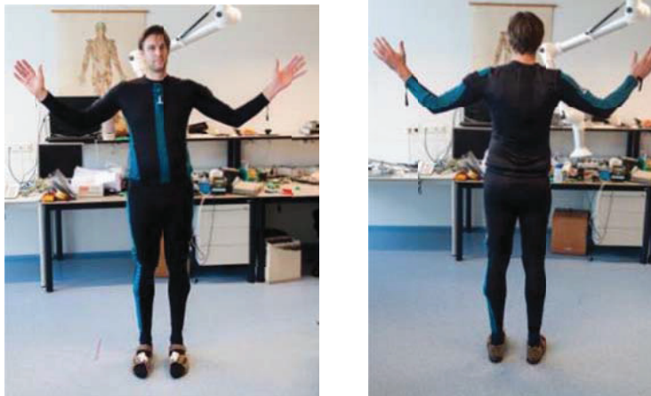
Figure 3. Prototype of the modular and wireless INTERACTION textile-integrated sensing system.
