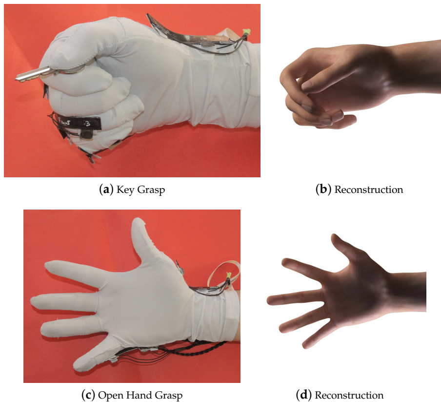
Figure 9. Comparison between real and reconstructed grasps (obtained from the five measurements extended to the 19-DOF pose and rendered in 3D Studio Max).
