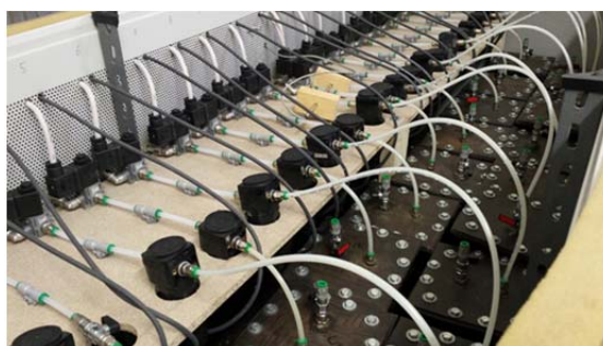
Figure 1: Scheme (left) and photo (right) of the experimental units used for anaerobic digestion tests. Each batch reactor has a gas inlet for flushing at the beginning of the assay (1), a compressed air filter (2), a T-pipe connector (3), a pressure transducer (4) and an opening controlled by an electrovalve (5).
