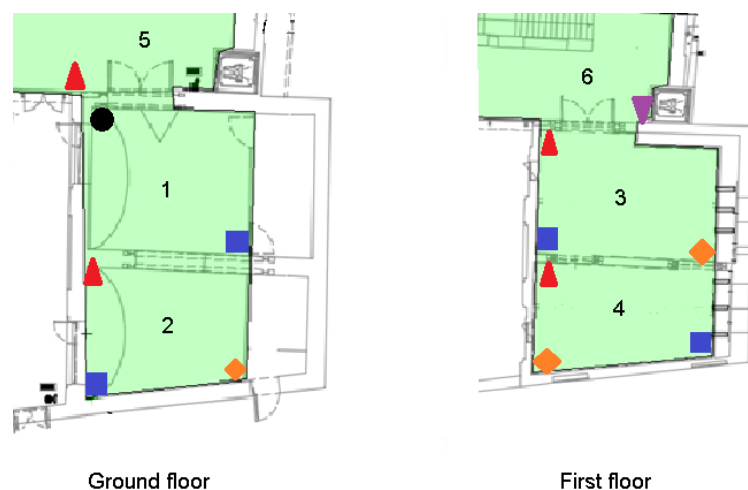
Figure A1. Sensor position in the four rooms. The round black marker identifies the QFA2001 sensor, the red triangle markers identify QAA24 sensors, the blue square markers identify 103AT-2 sensors (for the measure of temperature at 1.5 m and 2.5 m height), the orange diamond markers identify ZED-THL-M sensors, the inverted purple triangle marker identifies the 103AT-2 sensor for the measurement of temperature at 1.5 m height in the adjacent room.
