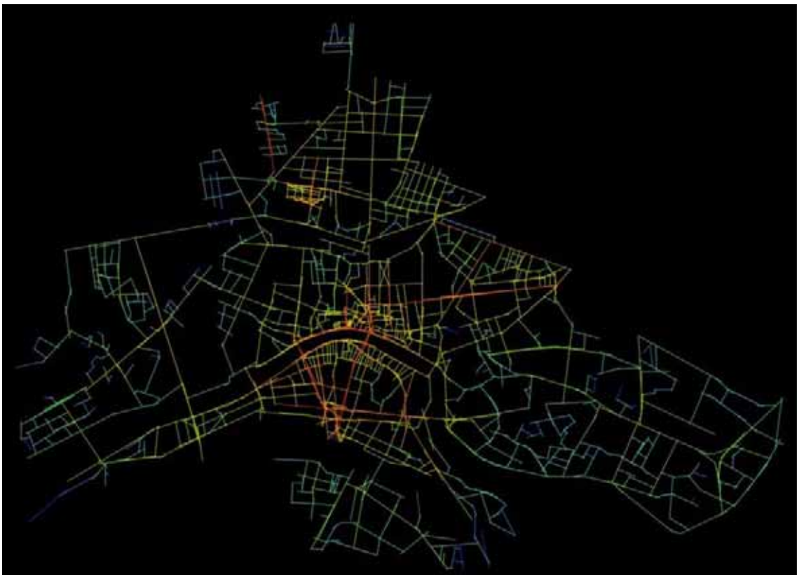
Fig. 8 The distribution of local (radius3) integration value in the lines of the axial map of Pisa
