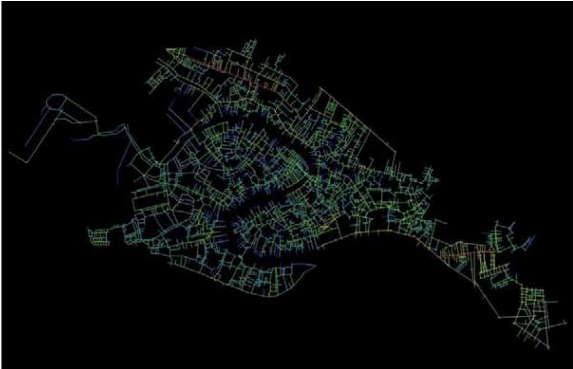
Fig. 9 The distribution of local (radius3) integration value in the lines of the axial map of Venice (without 'traghetti')
