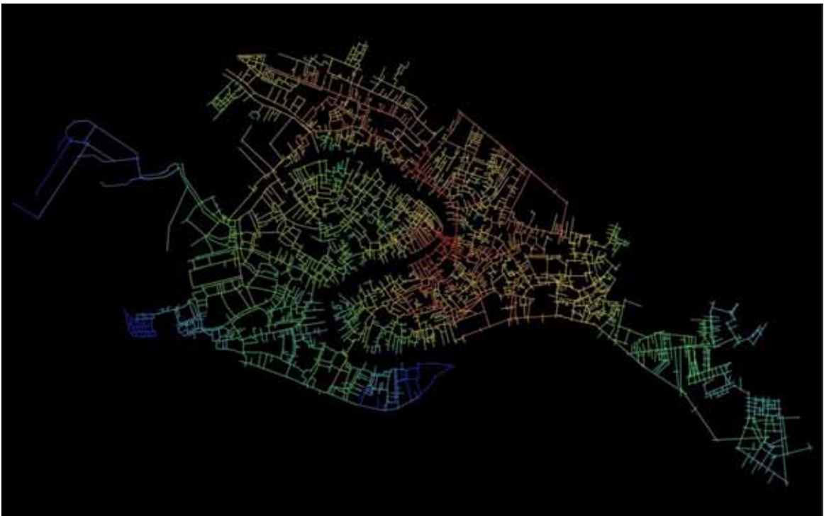
Fig. 6 The distribution of global integration value in the lines of the axial map of Venice (without 'traghetti')
