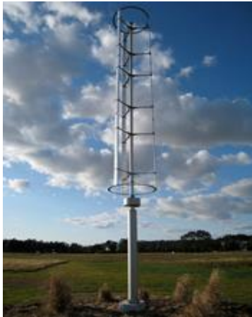
152 FIGURE 2: (left) Windspire 1.2kW VAWT; (right) comparison between experimental performance [7] and predictions obtained for 153 the Windspire turbine with ANSYS Fluent CFD software.
