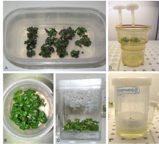
Fig. 1. Types of vessels used for the in vitro culture of sweet basil shoots: A - MicroboxECO 2 TM , B - PCCV25 TM , C - GA-7 box Magenta TM , D - temporary immersion system RITA TM , E - cylindrical bioreactor Growtek TM .
