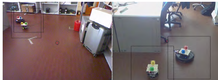
Fig. 7. Two cameras manage two robots at the same time.
