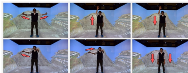
Figure 1: The gesture vocabulary. From left to right and top to bottom: 1) initiating measurement by stretching hands out 2) moving to a lower layer by raising the hand 3) moving to a higher layer by lowering the hand 4) Rotation of the right forearm from inside to outside for opening the contextual menu 5) closing the menu with an inverse movement 6) deselecting the current object with a sharp downwards movement of both hands.
