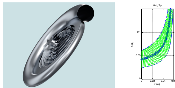
Figure 8. 3D rendering of the second sample of of centrifugal pump geometry (B, left) and meridional cross-section of the impeller (right).
