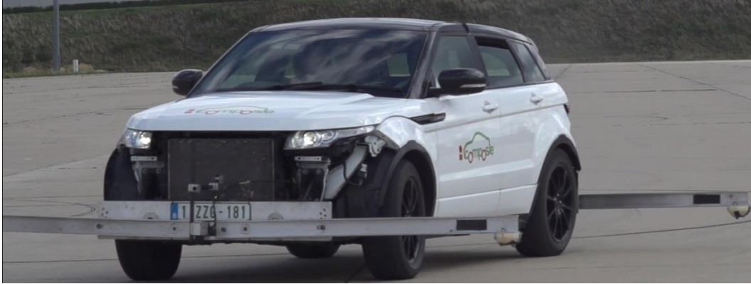
Fig. 1. The iCOMPOSE vehicle demonstrator: front view with the Corrsys Datron sensor installed across from the front bumper (Lommel Proving Ground, Belgium).
