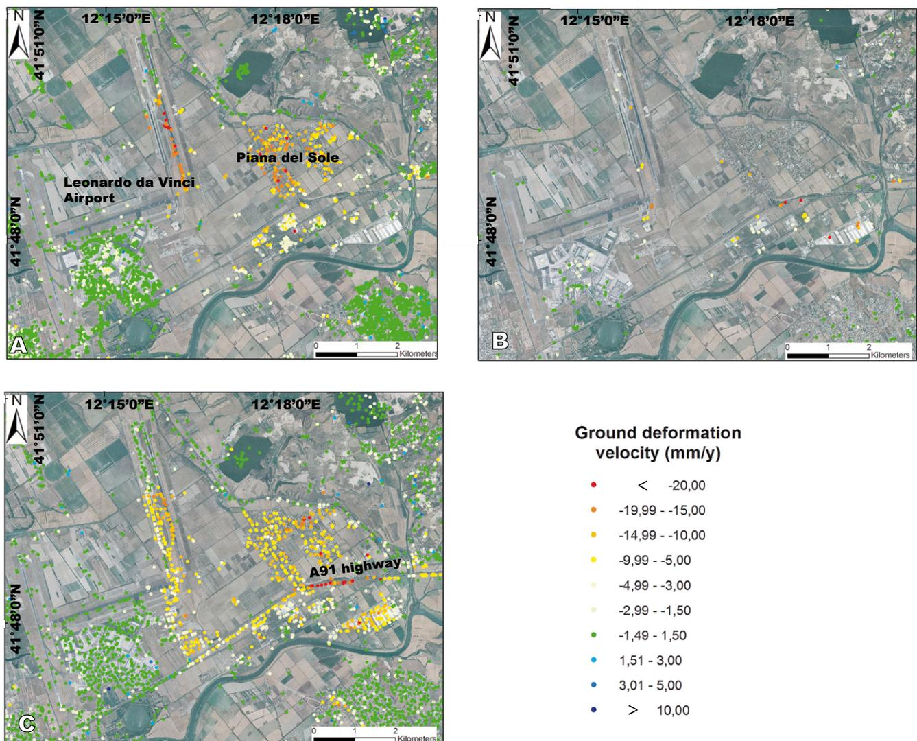
FIGURE 5. Ground deformation velocity maps in the area of Maccarese. A) ERS 1/2 (1992–2000); B) ENVISAT (2003–2005); C) RADARSAT-1 (2003–2006).
