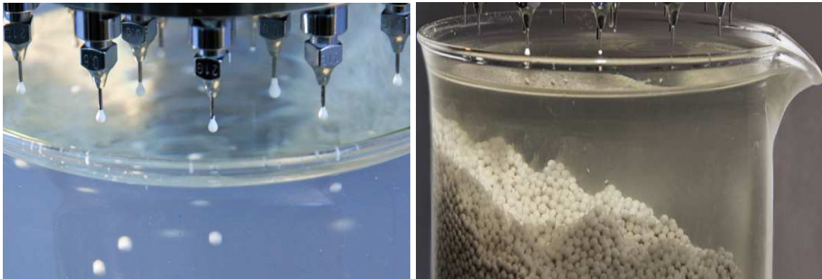
Figure 3: Drip casting process: cross linking in alginate gels involves cooperative bonding of divalent metal ions.
