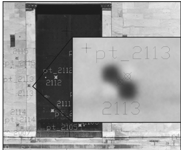
Figure 4 – Laser-computed and topographical targets on rectified image.
