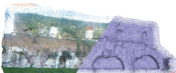
Figure 5 – Presence of cage projection on the textured model.
