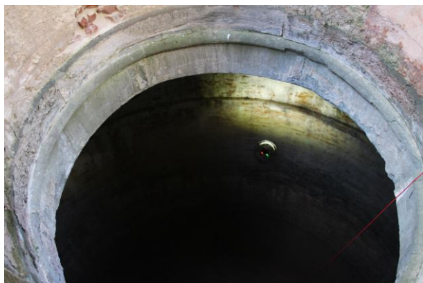
Figure 12 – Dark tank and UAV-borne lighting system.
