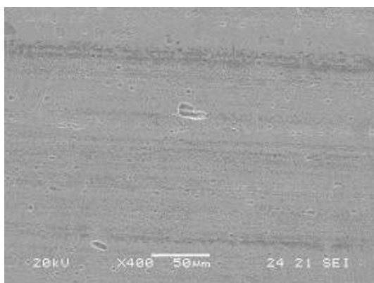
Fig. 15 Scanning electron microscope image of micro-pitted tooth.
