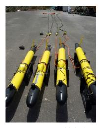
Figure 11. Folaga AUVs towing streamers with hydrophones.
