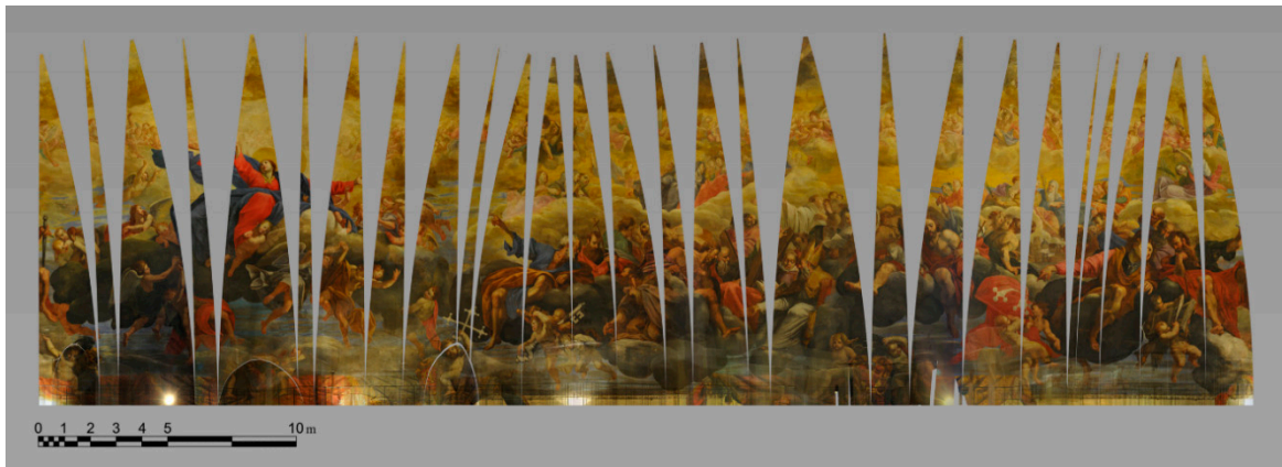
Figure 9. Pseudo-development by projection of the Pisa Cathedral dome.
