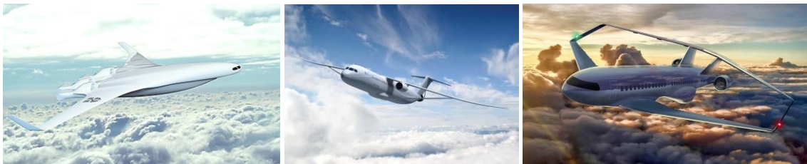
Figure 1: Concepts for Blended Wing Body from “Silent Aircraft Initiative” ([4]), Truss Braced Wings from “SUGAR” project ([5]) and PrandtlPlane from “PARSIFAL” project
